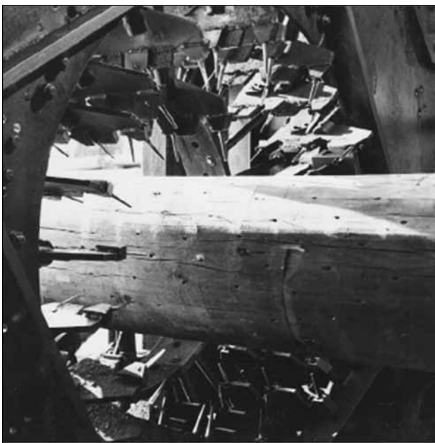
Figure 15-4. Deep incising permits better penetration of preservative.
