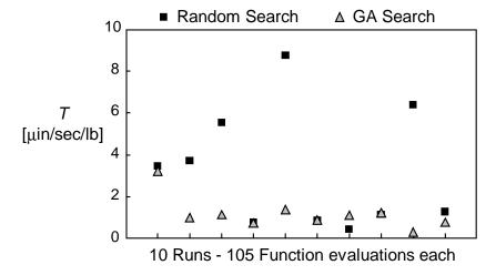
Figure 20 Comparison of genetic algorithm and random search results using the same number of function evaluations (105). Designs shown are the best found for each run.
