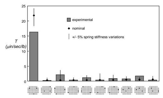
Figure 27 Experimental transmissibilities at 50 Hz of baseline and optimized designs, compared to analytical predictions.
