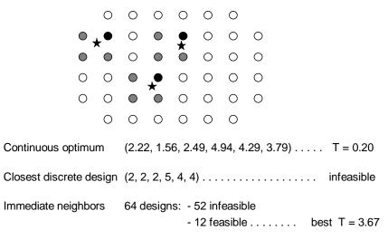
Figure 23 Results from continuous optimization and rounding.
