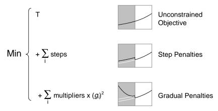
Figure 18 Penalty function approach used in this application; the shaded area is infeasible.
