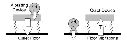
Figure 1 Vibration isolation systems.
