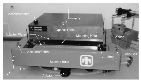
Figure 5 Experimental vibration isolation setup.
