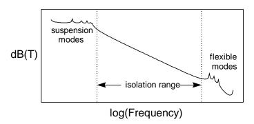
Figure 2 Typical transmission characteristics of isolation system.
