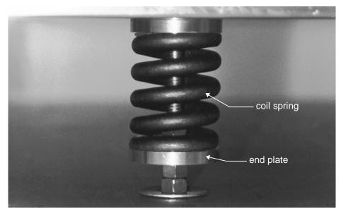
Figure 6 Steel spring isolator.
