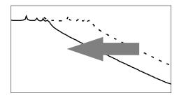
Figure 3 Improving isolation by softening the isolators.
