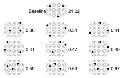
Figure 21 GA optimized designs and their transmissibilities at 50 Hz (in  $\mu$ in/sec/lb), compared to baseline configuration.
