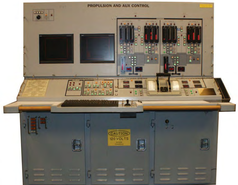
Figure 6-27 — Propulsion control system.
