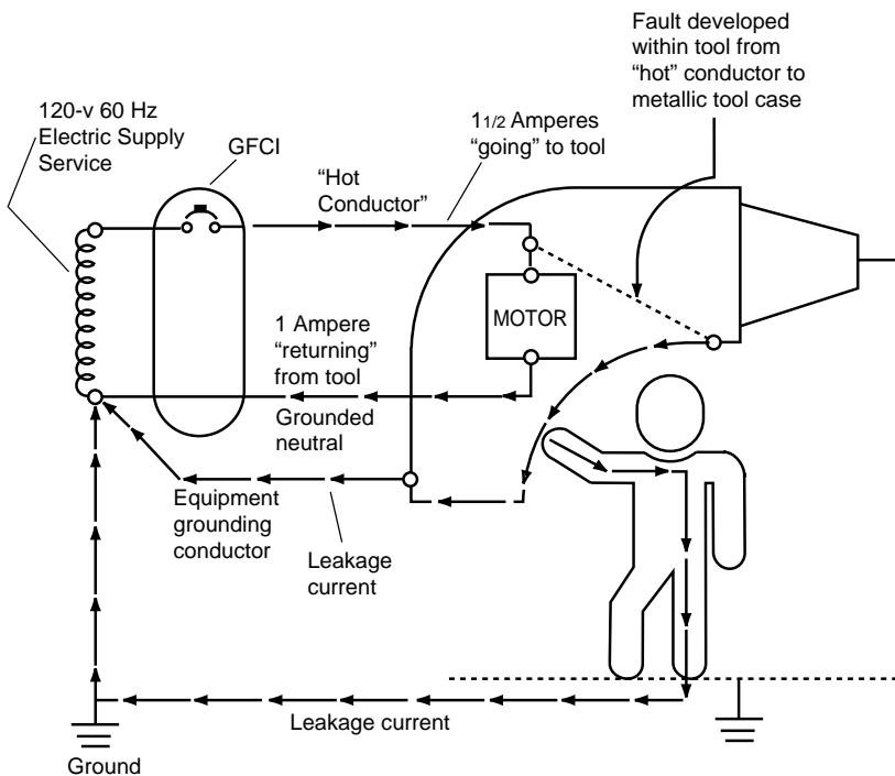
GFCI monitors the difference in current flowing into the "hot" and out to the grounded neutral conductors. The difference ( $\frac{1}{2}$  ampere in this case) will flow back through any available path, such as the equipment grounding conductor, and through a person holding the tool, if the person is in contact with a grounded object.
