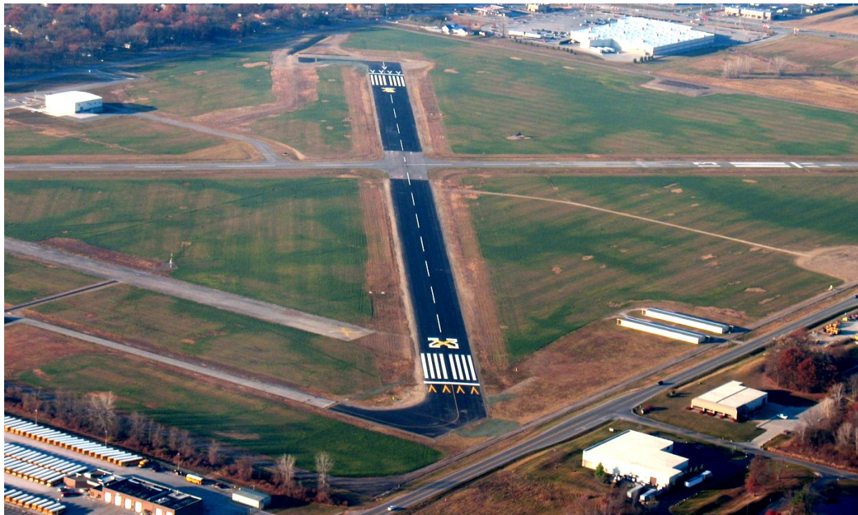
Figure 2-3. Markings for a Temporarily Closed Runway
