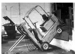
Forklift driven off loading dock.
