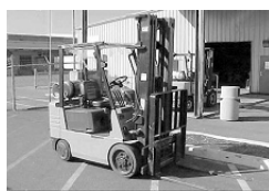
Safety features include an overhead guard.
