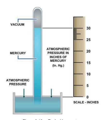
Figure 2-12 — Typical barometer.
