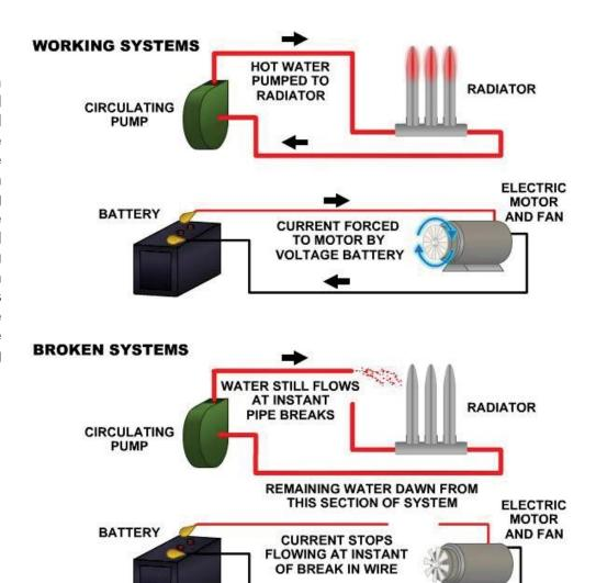
Figure 2-3 — Different characteristics of current and water.
