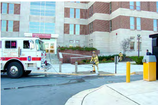
Figure 2.7. During initial operation at this structure, the first arriving engine crew is already using a fire lane, a fire hydrant, the fire department connection, and the key box. Interior operation will soon involve the alarm system, stairs, standpipe system, and other building features.
