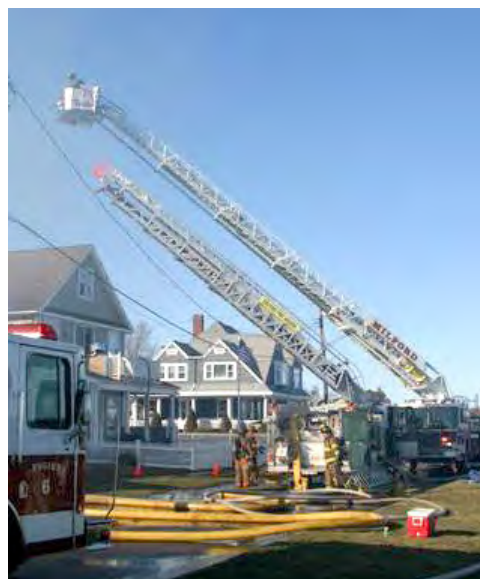
Figure 2.6. Two types of fire service aerial apparatus — one with a straight ladder (left) and the other with an elevating platform (right). The latter type of aerial apparatus is often referred to as a “tower”, “tower truck”, or “tower ladder”.
