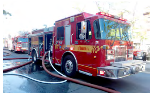
Figure 2.4. A pumper operating at an incident. The red hose is supplying water from a fire hydrant to the pumper. The white hose is a fire attack line.
