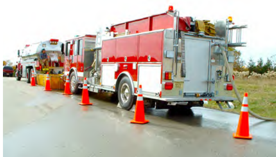
Figure 4.3. A rural water supply operation. The water tender on the left is filling the yellow portable basin. The pumper on the right is drafting water from that basin to feed hose lines.
