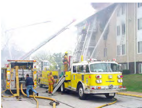
Figure 3.1. An apartment fire where the fire apparatus access was adequate width and a proper distance from the building.
