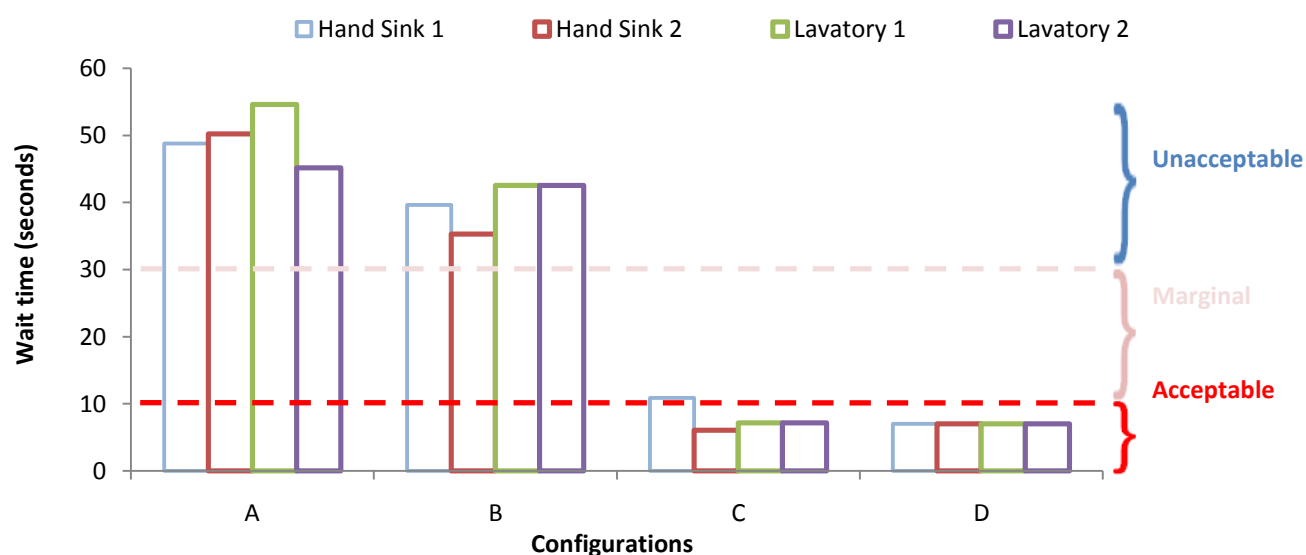
Figure 43. Estimated initial wait time for hot water at hand washing sinks.
