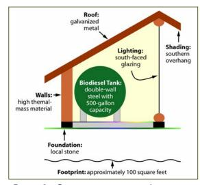
Figure 3. Green construction techniques can be integrated into BMPs for small structures used to store field equipment or to house treatment components such as pump equipment.
