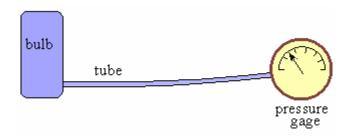
Suppose the gas inside the bulb and tube can be considered an ideal gas. The ideal gas law is:
