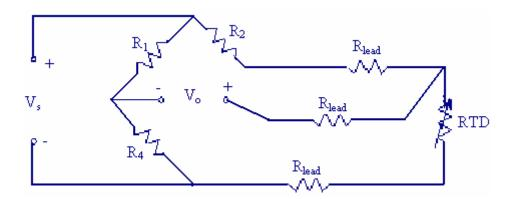
It is still a quarter bridge circuit, since only one of the four bridge resistors has been replaced by the RTD. However, one of the lead wires has been placed on the  $R_2$  leg of the bridge instead of the  $R_3$  leg.
