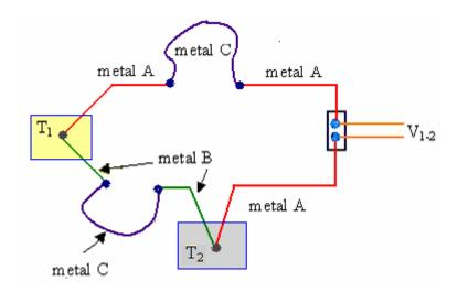
Again, if the two new junctions (this time between metals A and C) are at the same temperature, there is no net effect on the output voltage.
