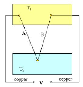
With enough sensing junctions, a thermopile can actually generate a useful voltage. For example, thermopiles are often used to control shut-off valves in furnaces.
