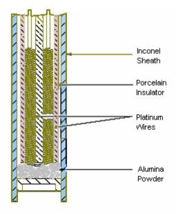
Internal Construction of Typical RTD
