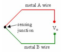
The voltage is measured to infer the temperature. In practical operation, wires A and B are connected to a digital voltmeter (DVM), digital multimeter (DMM), digital data acquisition system, or some other voltage measuring device. If the measuring device has very high input impedance, the voltage produced by the thermo-junction can be measured accurately.
