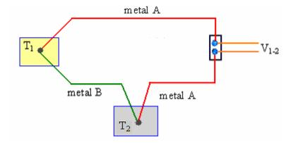
The law of intermediate metals states that the voltage reading,  $V_{1-2}$  does not change if one adds a third (intermediate) wire in line with any of the wires in the circuit, as sketched below:
