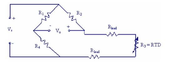
R<sub>lead</sub> represents the resistance of one of the wires (called *lead wires*) that run from the bridge to the RTD itself. Lead resistance was of no concern in strain gage circuits because R<sub>lead</sub> remained constant at all times.
