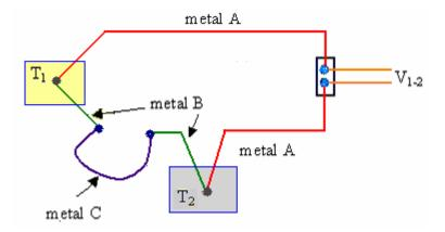
In the above diagram, it is assumed that both of the new junctions (between metal B and metal C) are at the same temperature, i.e. ambient temperature,  $T_a$ .
