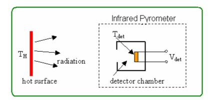
The detector itself is usually a thermopile. It measures  $T_{det}$ , the temperature of the detector inside the chamber.  $T_{ind}$  is the *indicated* temperature, which is calculated from  $T_{det}$ , from the known geometry and the radiation equations.  $T_{ind}$  is calibrated as a function of  $T_H$  for a body of some assumed emissivity.
