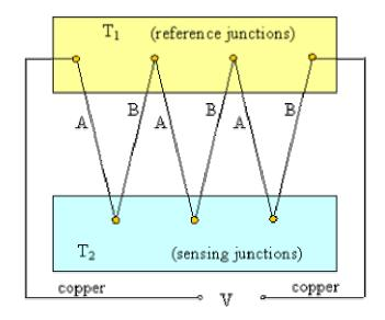
As T<sub>2</sub> is increased, the output voltage increases significantly. The advantage of a thermopile (as compared to just one sensing junction) is *increased sensitivity*.
