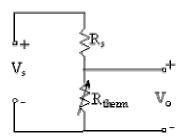
From the circuit diagram, it is clear that this is a simple voltage divider.  $R_s$  is some fixed (supply) resistor.  $R_s$  and the supply voltage,  $V_s$ , can be adjusted to obtain the desired range of output voltage  $V_o$  for a given range of temperature.
