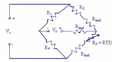
In the above diagram, it is clear that if  $R_{lead}$  changes equally in leg 2 and leg 3 of the bridge, its effect cancels out.
