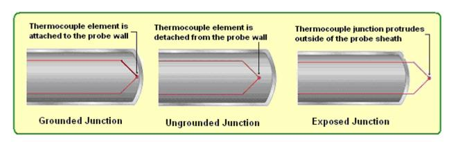
In summary, the exposed junction provides the quickest response time followed by grounded junction. Temperature measurement decisions can make or break the expected results of the process. Choosing the correct sensor for the application might be a difficult task, but processing that measured signal is also very critical.
