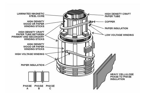
Figure 2 – Transformer Construction.
