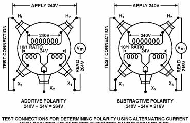
TEST CONNECTIONS FOR DETERMINING POLARITY USING ALTERNATING CURRENT WITH REDUCED VOLTAGE FOR EXCITATION ON THE PRIMARY SIDE. (NOTE THAT THE POSITION OF  $X_1$  AND  $X_3$  ARE REVERSED)
