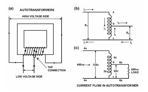
Figure 9 – Autotransformers.
