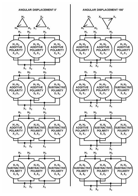
Figure 18 – Delta-Delta Connections, Single-Phase Transformers for Three-Phase Operation.
