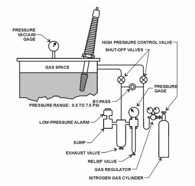
Figure 24 – Typical Transformer Nitrogen System.
