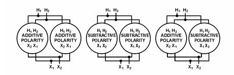
Figure 16 - Single-Phase Paralleling.
