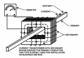
Figure 12 - Current Transformer.
