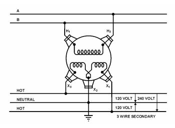
Figure 15 – Single-Phase Transformer.
