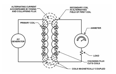
Figure 3 – Transformer Action.
