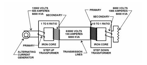
Figure 5 – Step-Up and Step-Down Transformers.
