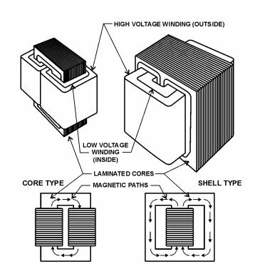
Figure 6 – Magnetic Circuits.
