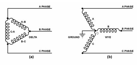
Figure 17 – Three-Phase Connections.
