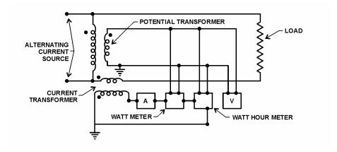
Figure 10 – Connections of Instrument Transformers.
