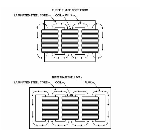
Figure 7 – Three-Phase Core Form and Three-Phase Shell Form Transformer Units.
