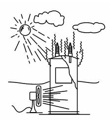
free circulation of oil through the core and coils; warmer and lighter oil rises to the top of the tank, cooler and heavier oil settles to the bottom. Several methods have been developed for removing heat that is transmitted to the transformer oil from the core and windings (figure 21).
