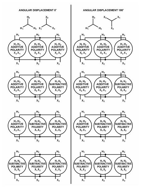
Figure 19 – Wye-Wye Connections, Using Single-Phase Transformers for Three-Phase Operation.
