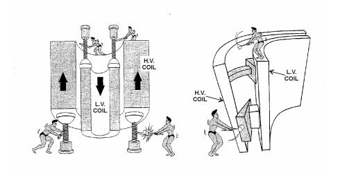
Figure 8 – Transformer Internal Forces.
