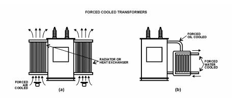
Figure 22 – Forced-Air/Oil/Water-Cooled Transformers.
