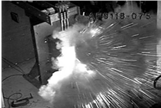
Figure 1.3: Simulated arc-flash incident, conducted at 250V, 44 KA (44,000 amps). Energy intensity: 8.48 Cal/cm 2 .
