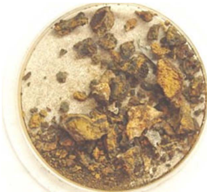
Large Rust Particles
