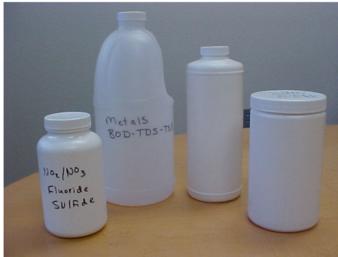
NO 2 /NO 3 , Fluoride, Sulfide, Metals, BOD-TDS-TSS Wide-mouth Sludge/Metals bottle.
