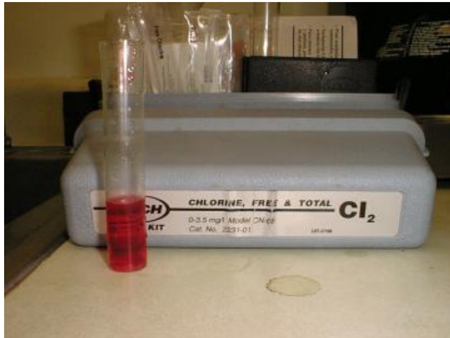
Simple DPD Chlorine Field Test Kit.
