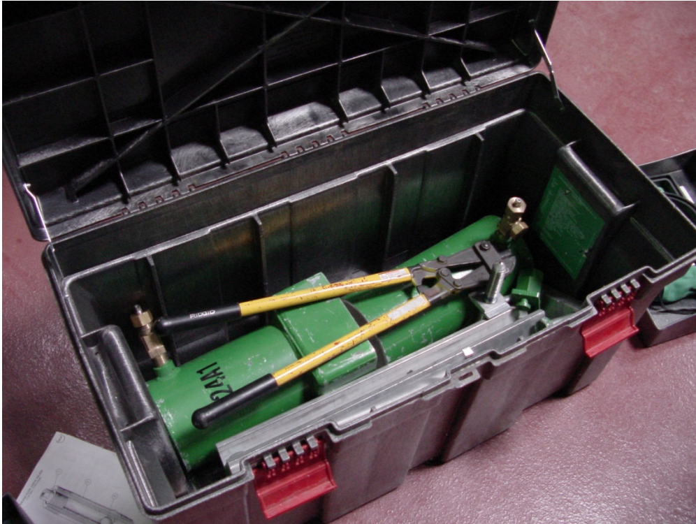
Chlorine C repair kit, used for the tank cars and tankers.
