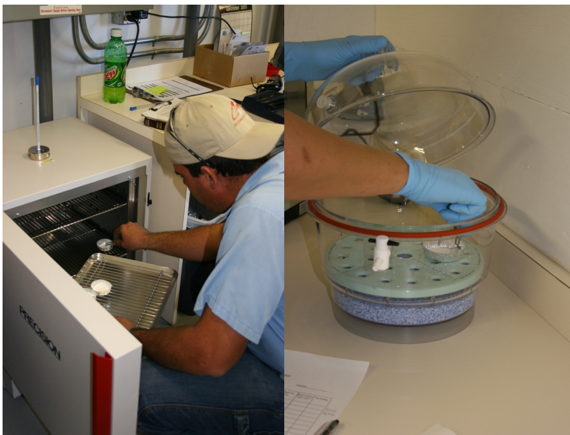
Top left, filters being baked at 105°C. Right photograph, filters in desiccant. Bottom photograph, preparation for the fecal test.
