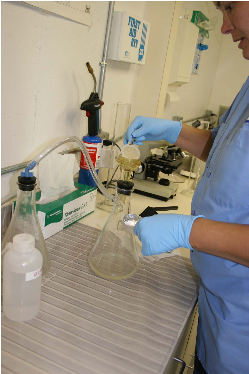
Lab tech removing filter for TSS analysis.
