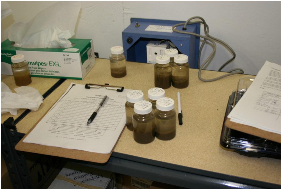
Operators analyze sludge samples to improve wasting.
