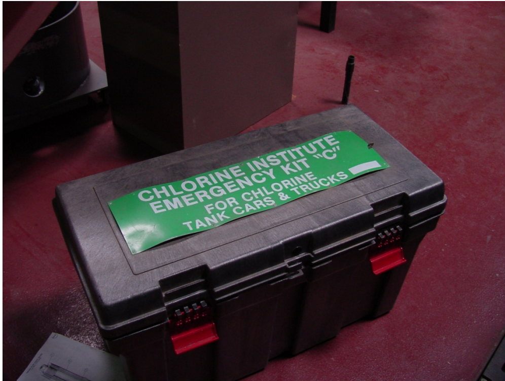
Chlorine C repair kit, used for the tank cars and tankers.
