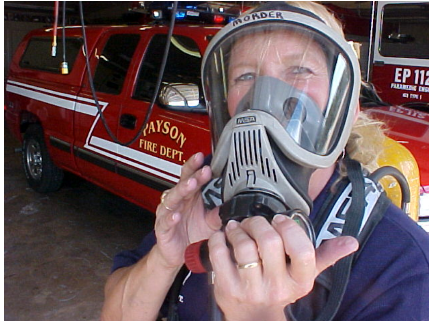
SCBA Fit Test, insuring an air tight fit.
