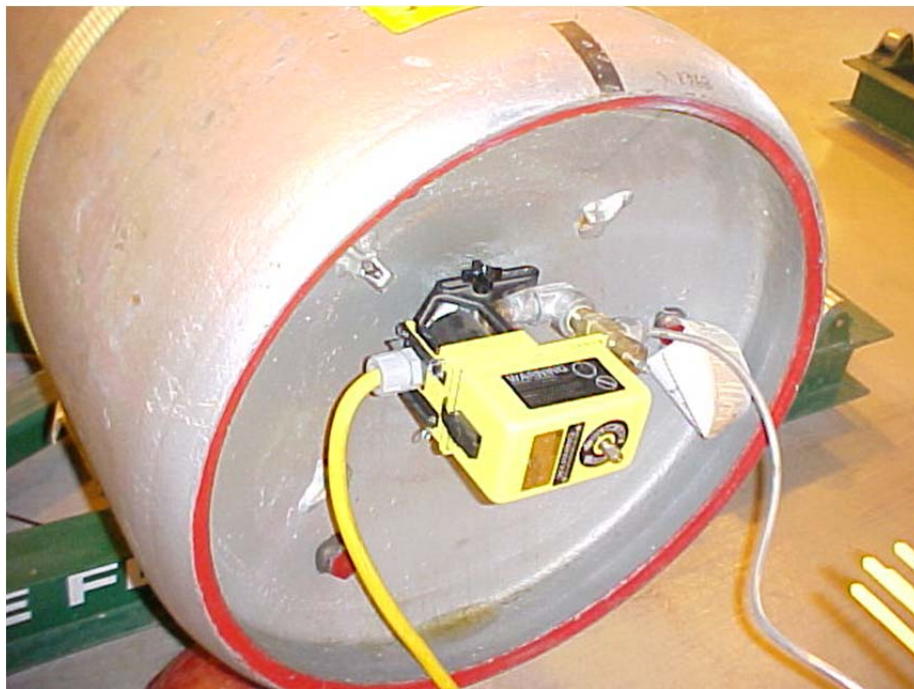
1-ton chlorine gas container with an automatic leak detection and shut-off device.
