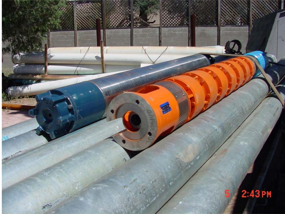
A new 8 inch submersible pump and motor with 6 inch column pipe about to be installed in a high capacity municipal supply well.
