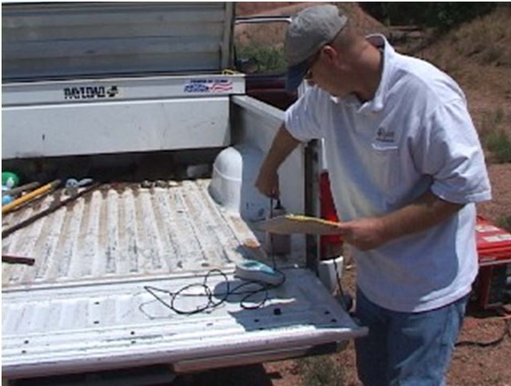
The inspector is using a pH meter to check a grab sample.
