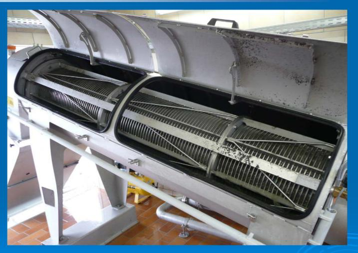
Inclined Screw Press with skin removed showing the wedge wire basket and spray bar
