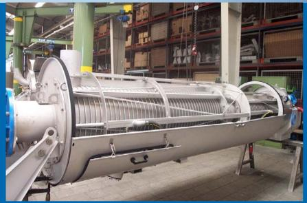
⇒ Screw Press with skin removed showing the wedge wire baskets
