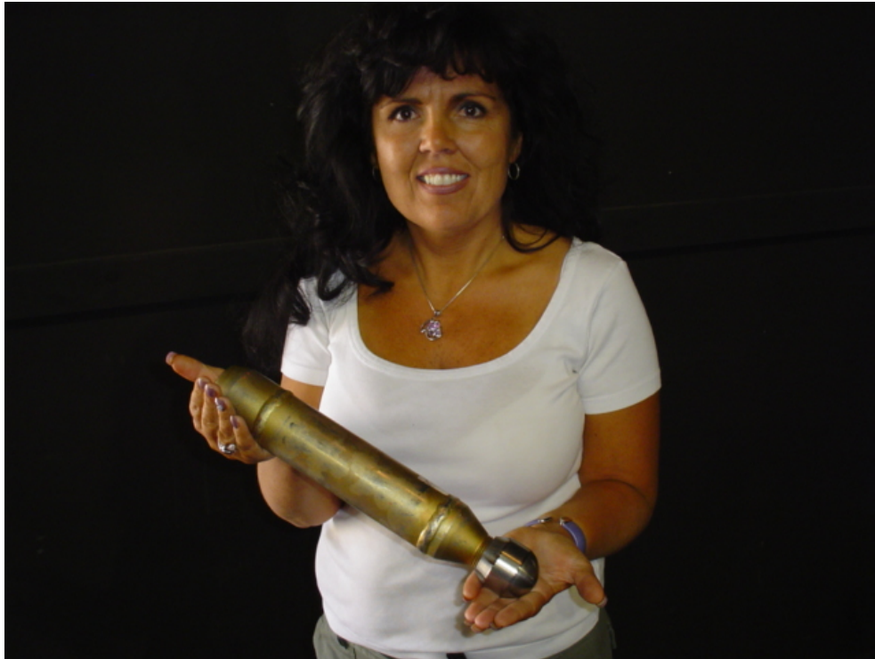
Course author and wastewater collection expert, Melissa Durbin with a hydraulic sewer cleaning head and various root cutting devices for use on a rodder. If you need any assistance, please call me or our staff.
