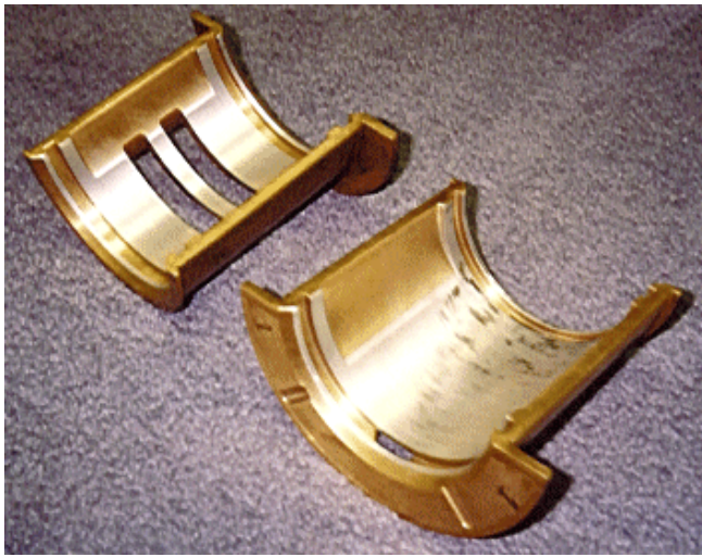
Figure 4.31: Lubrication Holes and Grooves in Plain Bearings
