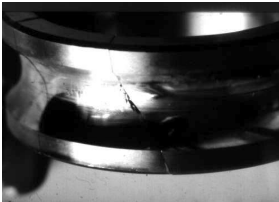
(a) Cracked Race due to too much Interference
