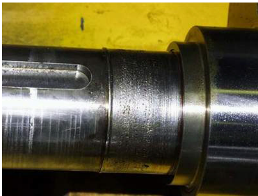
(c) Fretting on Shaft due to Loose Fit between Shaft and Bearing
