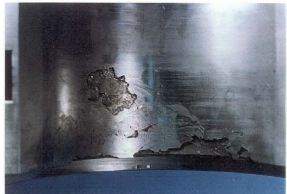
(b) More Advanced Fatigue Damage
