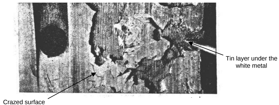
(c) Severe Fatigue Damage
