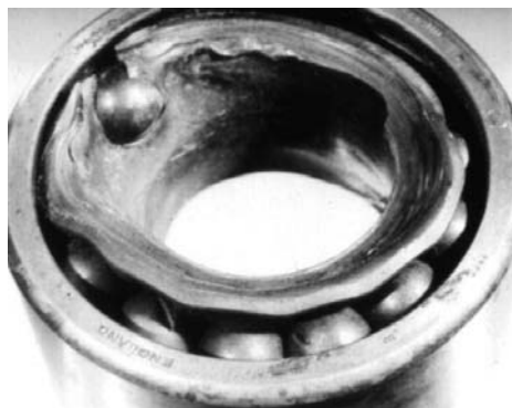
Figure 7.15: Bearing Seizure Damage
