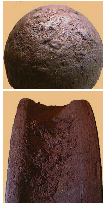
Figure 4.27: Badly Corroded Ball and Race
