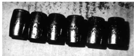
(b) Fatigue Damage on Spherical Rollers
