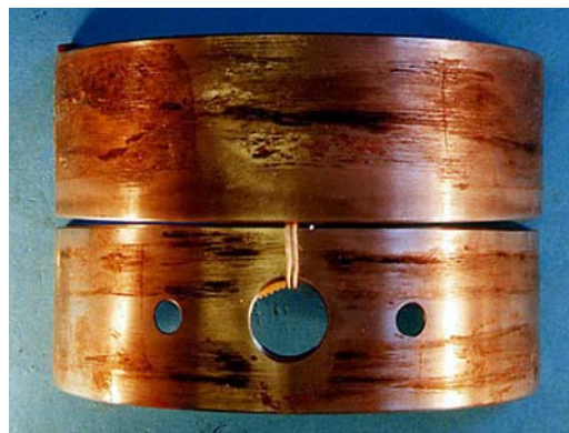
Figure 5.9: Fretting Due to too Little Interference between Shells and Housing
