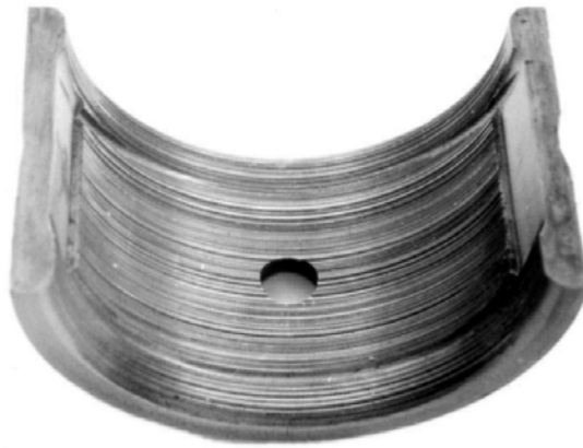
Figure 5.3: Heavy Scoring of a Lead-bronze Journal Bearing
