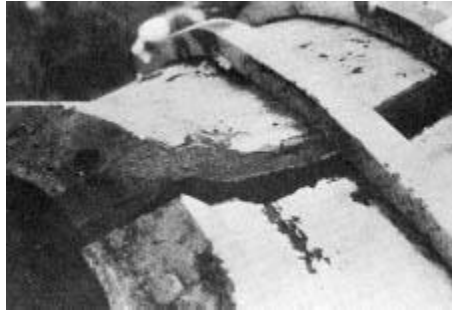
Burst pipe in power station Big Creek #3, USA
