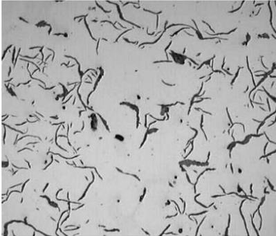
Photomicrograph showing graphite form in gray iron.
