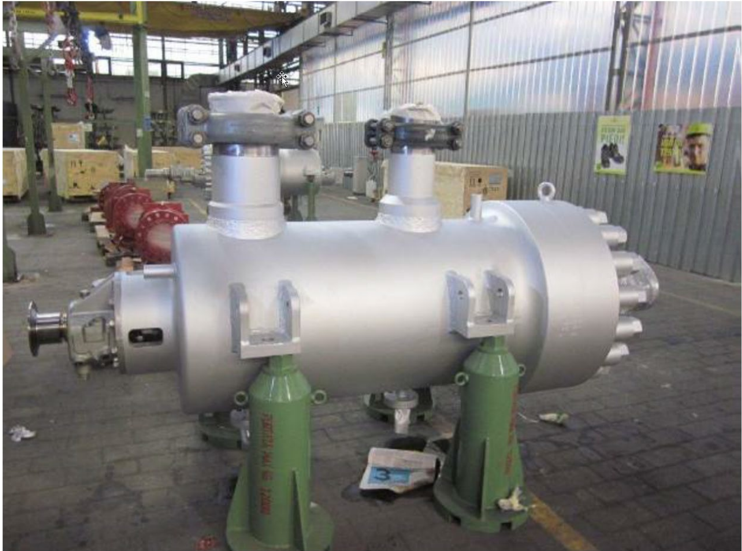
13-PU103 common spare pump for 13-PU101/102 – final inspection at GE, Italy, Dec-2013
