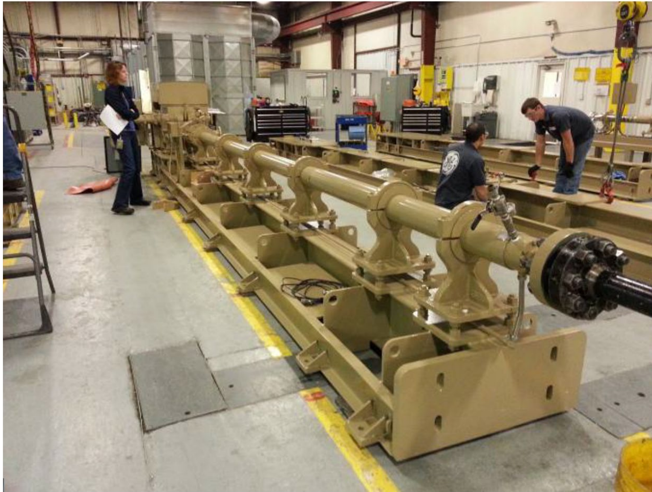
12-PU108A/B – HP Wash Water Pumps – 300hp, 176 bar P-disch – on test at GE Wood Group, Tulsa, OK, USA, Dec-2014
