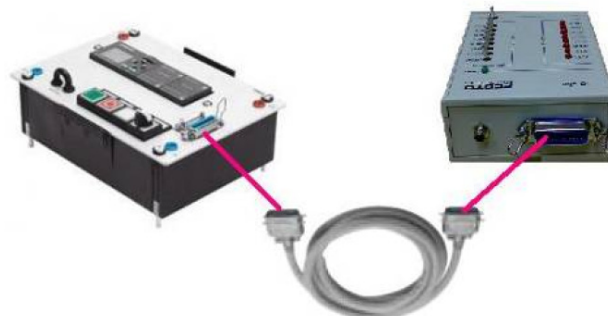
Fig 2.21 Connecting IO Simulator to LOGO!
