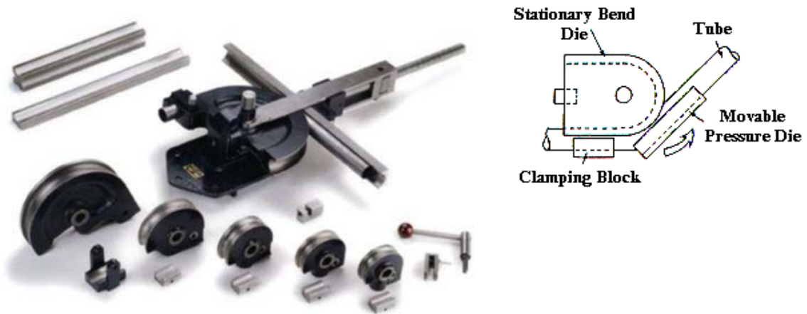
Figure 6.5: Compression Pipe Bender
