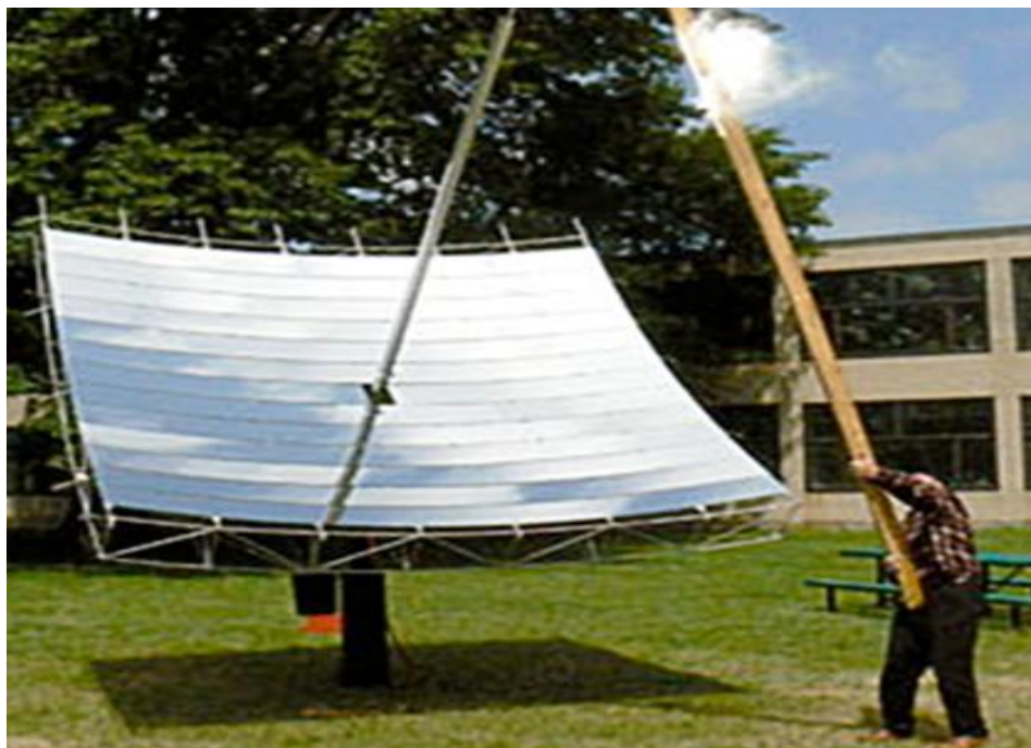
Fig. 16: Parabolic trough solar collector
