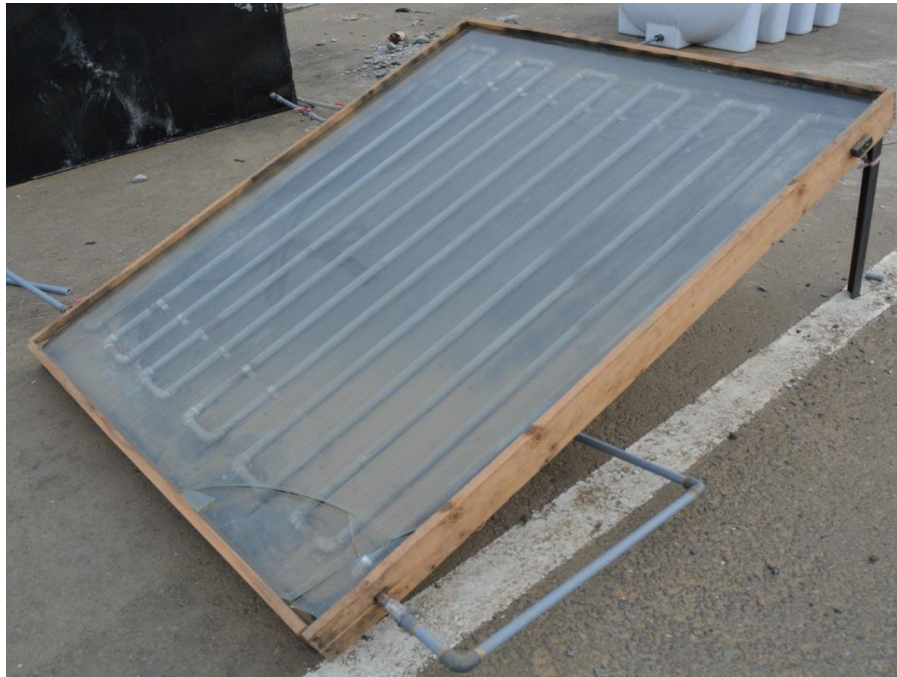
Fig. 32: Present flat plate solar collector
