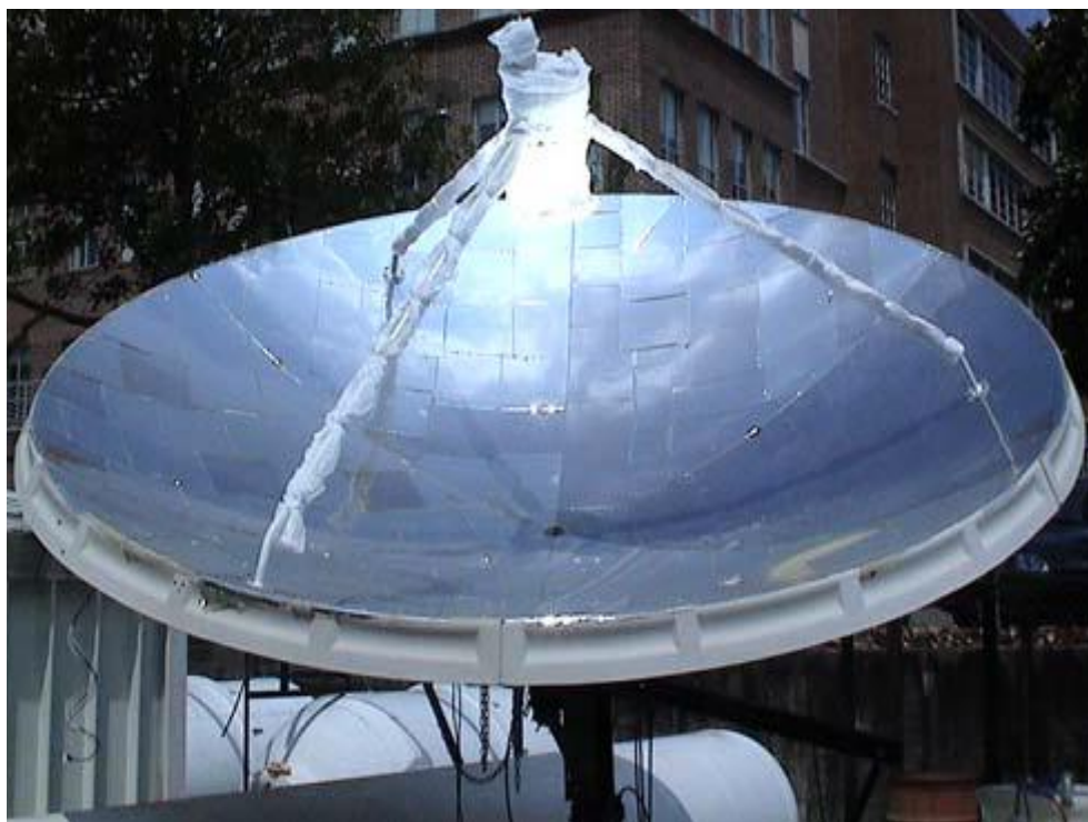
Fig. 17: The concentrator Fresnel mirror solar collector
