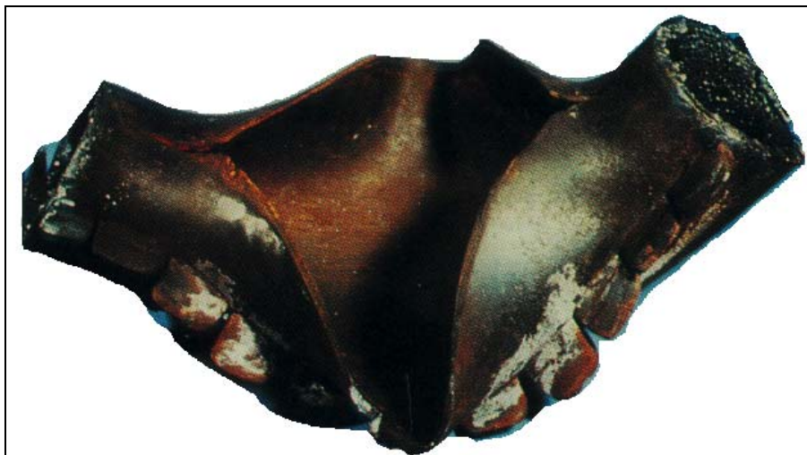
Figure 6. Extreme Short Term Overheating
