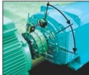
The EASY-TURN™ Program requires only 40° of rotation for an alignment solution.
