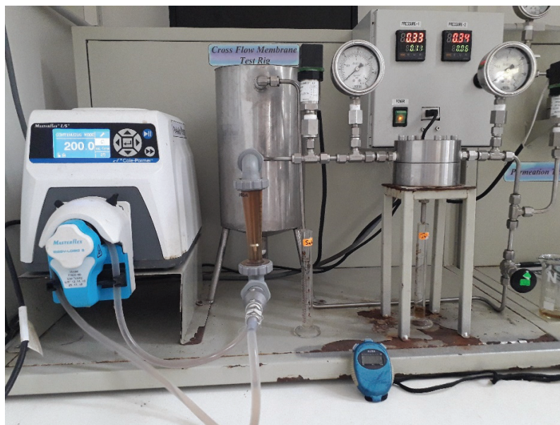
Figure 3. CFR test configuration (filtration treatment set).
