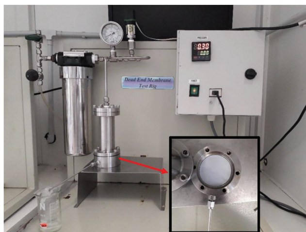
Figure 4. Dead-end test (pure water permeation set-up).
