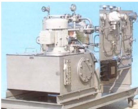
High pressure system designed to lubricate and cool seals in oil field export pumps in a tropical climate
