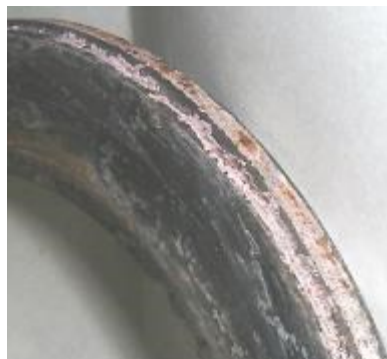
Cobalt bonded tungsten carbide mating ring showing results of sea water attack
