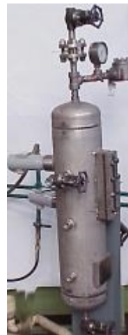
API 682 System with threaded connections
