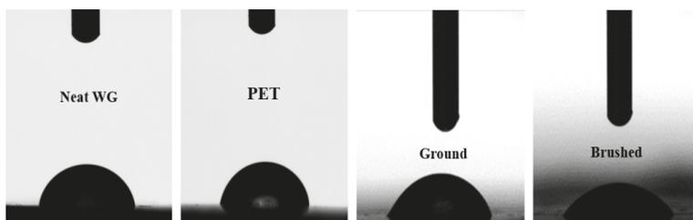
**Figure 12.** Water droplets on the samples during the goniometer test.
