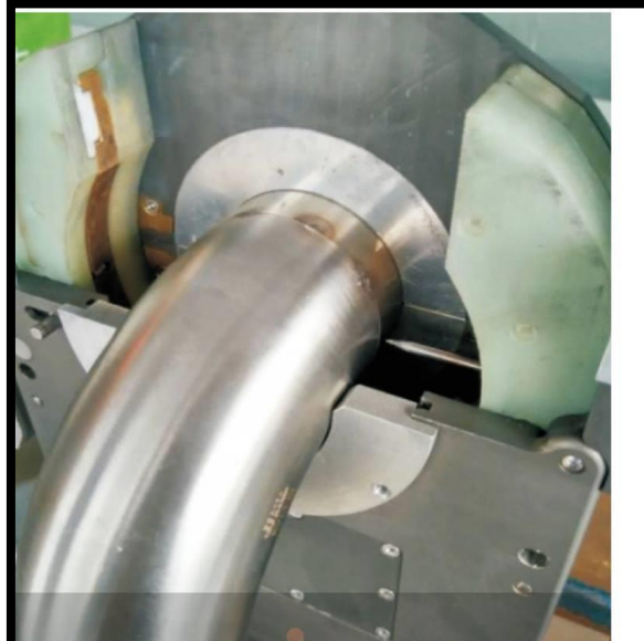
Orbital Welding Machine Enclosed Weld Head for Purified Water Treatment
