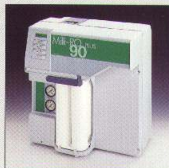
Millipore Milli-RO Plus Reverse Osmosis Systems are available for 6 l/h (left) to 90 l/h (right) of purified general laboratory grade water.
