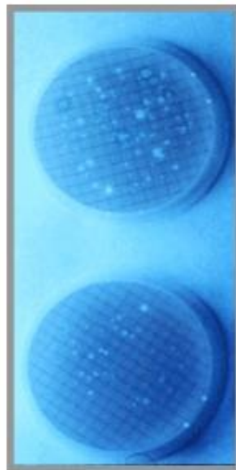
Total coliform colonies fluoresce under long-wave UV light.
