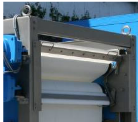
Filter cake discharge
