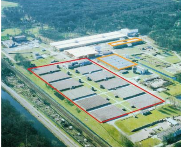
Figure 33 - Difference in surface area between rapid filtration and slow sand filtration
