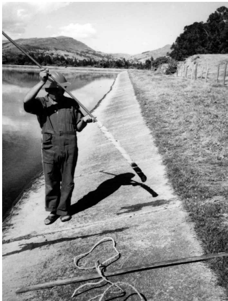
Figure 1 Sludge Depth Measurement by the 'White Towel' Test
