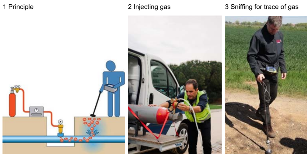
Figure 36 Gas injection leak detection technique (Sources: Primayer (1, 3), EPAL (Lisbon) (2)).
