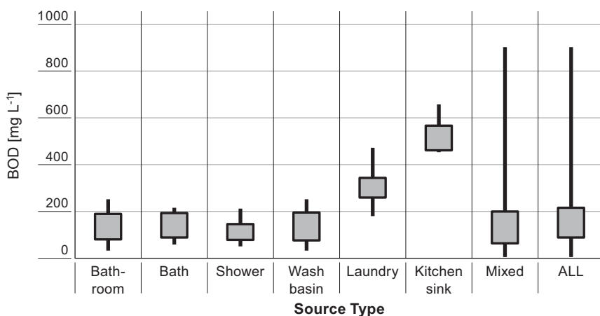
Figure 19.1 Reported ranges in organic strength for different greywater sources. The box shows the range between the 25 and 75 percentiles, the lines show the complete data range. Based on a comprehensive internal review of literature values.
