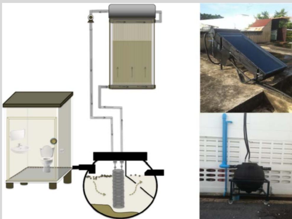
Figure 3.3 Field testing of the solar septic tank at the Asian Institute of Technology, Thailand (Source: AIT 2015).
