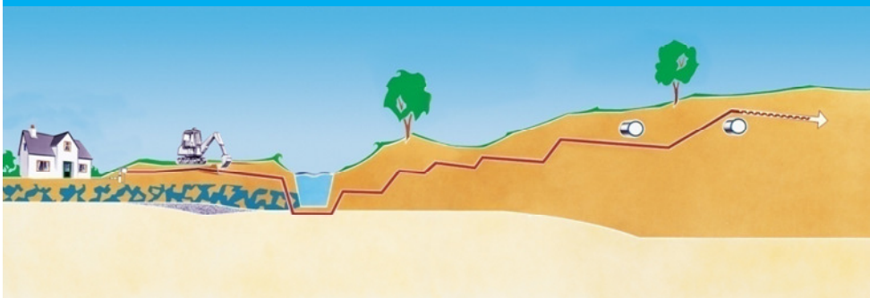
Vacuum sewer system
