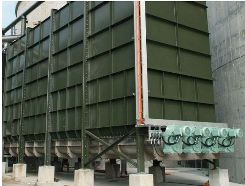
Figure 15: Rectangular Hopper with Live Bottom Screw Conveyors (courtesy of Asdor)
