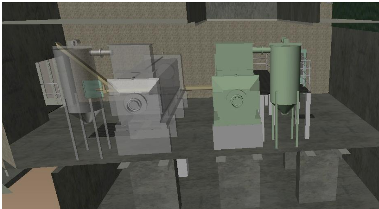
Figure 16: Section View (Looking North) of Conceptual Layout of FKC Screw Press in Centrifuge Room
