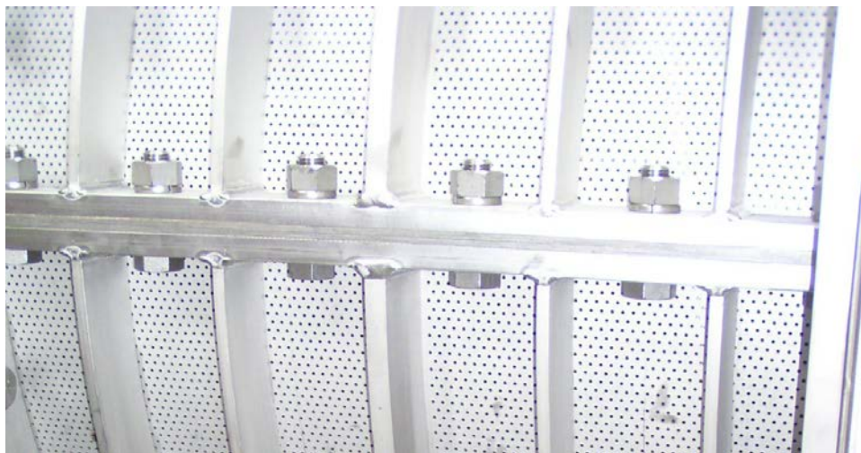
Figure 5: Typical Screw Press Screen
