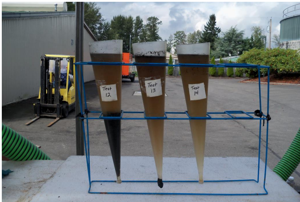
Photo: of centrate increasing the differential speed from left to right. The numbers represent the test runs during the demonstration.
