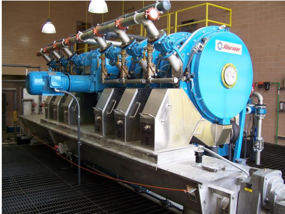
Figure 9: Multi-Channel Rotary Press (courtesy of Fournier Industries)
