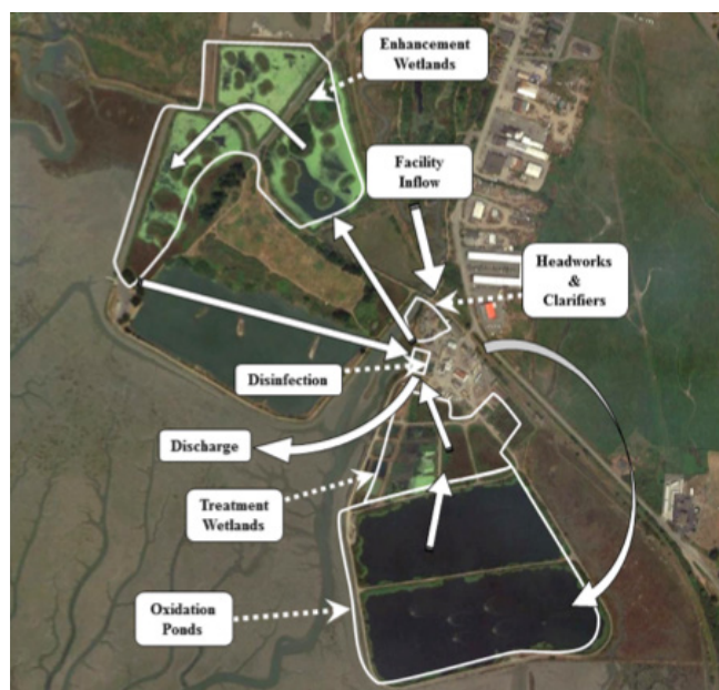
Figure 2: The flow pattern for the City of Arcata wastewater treatment plant and TW is complex. All processes are basically at the same elevation and are widely distributed, which requires several pump stations.
