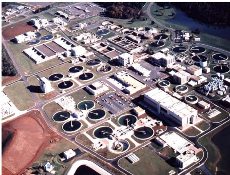
**Figure 27.3** Aerial photo of a portion of the 204,400 m<sup>3</sup>/d (54 MGD) UOSA water reclamation plant known as the Millard H. Robbins, Jr. Water Reclamation Facility.
