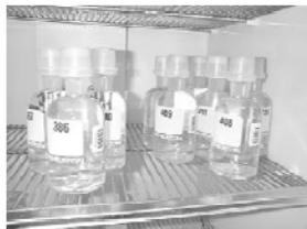
Incubated at 20 \pm 1^\circ \text{C} for 5 days in the dark
