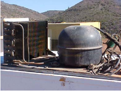
Example of a compressor unit from a refrigeration unit. The Freon will be reclaimed before this unit is recycled for scrap metal.
