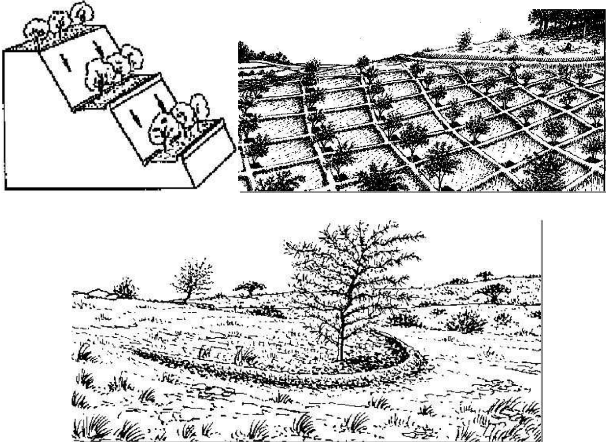
Figure 9 Examples of micro-catchment water harvesting (contour bench terrace, bunds, Negarim system) (Source: FAO, 1999)
