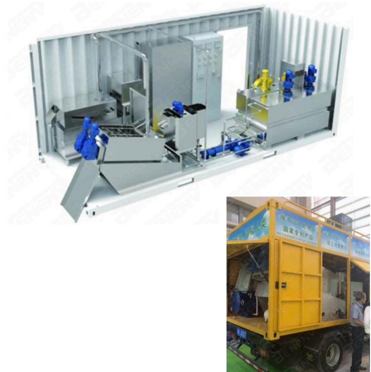
Figures (Top to Bottom): Interior of mobile screw press;
