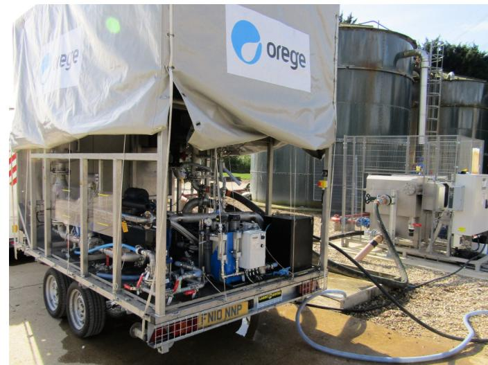
Figure: Orege Mobile Thickening Unit, SLG—Source: [LinkedIn](#)
