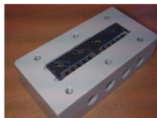
Figure 6.15 Photographs of the chip-half with the electrodes for the Hybridization-chip (left) and the hybridization chip mounted in its holder (right).
