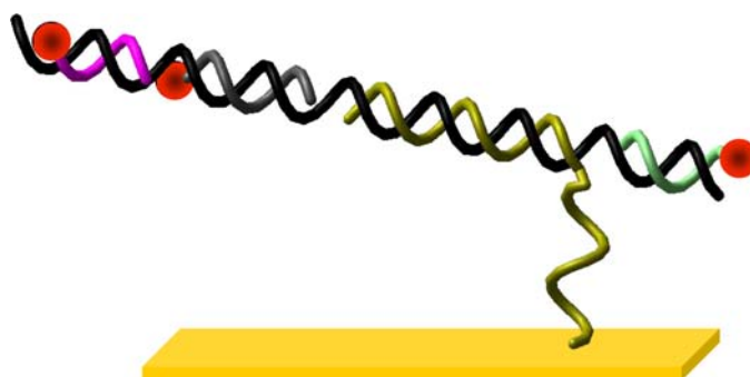
Scheme 8.2 Schematic representation of the binding and labelling of a ss-RNA or DNA (long black strand) by a surface-tethered oligonucleotide, with subsequent (singular or multiple) labelling by oligonucleotides bound to alkaline-phosphatase (represented as a sphere).
