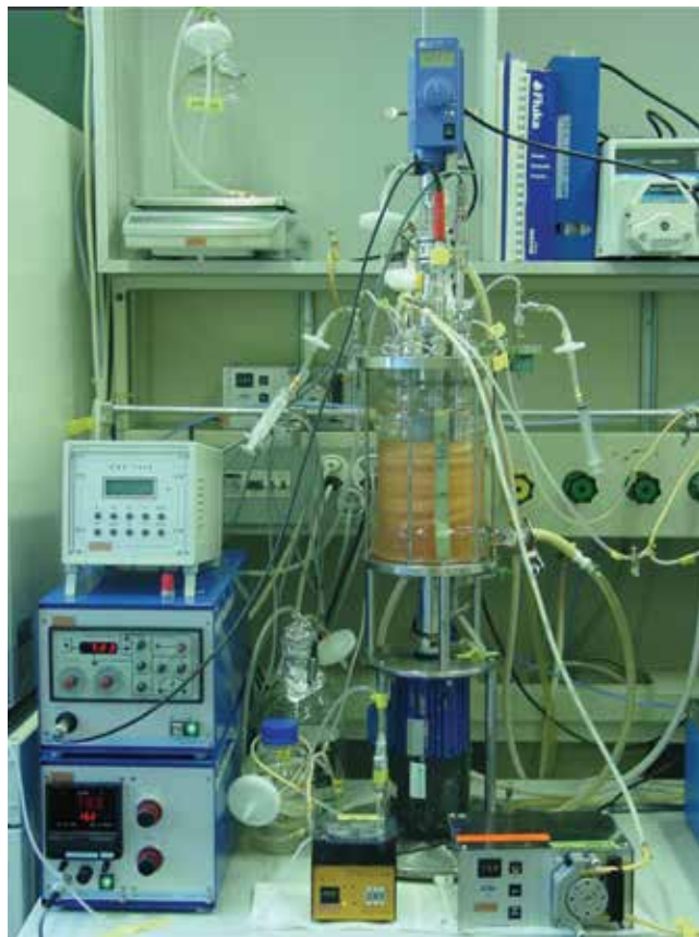
▲ Figure 4. Mammalian cell culture in a bench-scale bioreactor.
