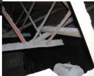
◀ Figure 8. Two workers went to inspect a bucket-elevator motor, which happened to be surrounded by piles of iron dust. During motor restart, vibrations dispersed powder on the floor and equipment. The dust ignited and created a flash fire, killing both workers. Source: (8).
