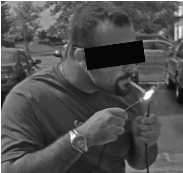
Figure 2.5 Dangerous dc arc-fault (do not try this at home) Smoking kills
